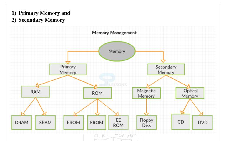
**Primary Memory:** - It is also called as the main memory of the computer. It stores the instructions, operating system and data which required to run the computer. There are two types of primary memories.
