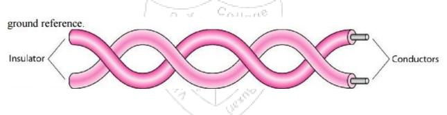
The most common twisted-pair cable used in communications is referred to as unshielded twisted-pair (UTP). IBM has also produced a version of twisted-pair cable for its use called shielded twisted-pair (STP). STP cable has a metal foil or braided mesh covering that encases each pair of insulated conductors. Although metal casing improves the quality of cable by preventing the penetration of noise or crosstalk, it is bulkier and more expensive.
