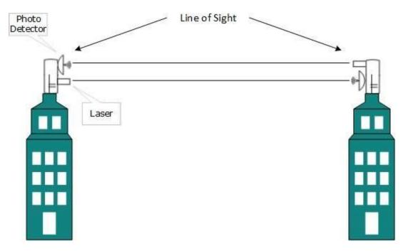
Laser works as Tx (transmitter) and photo-detectors works as Rx (receiver).
